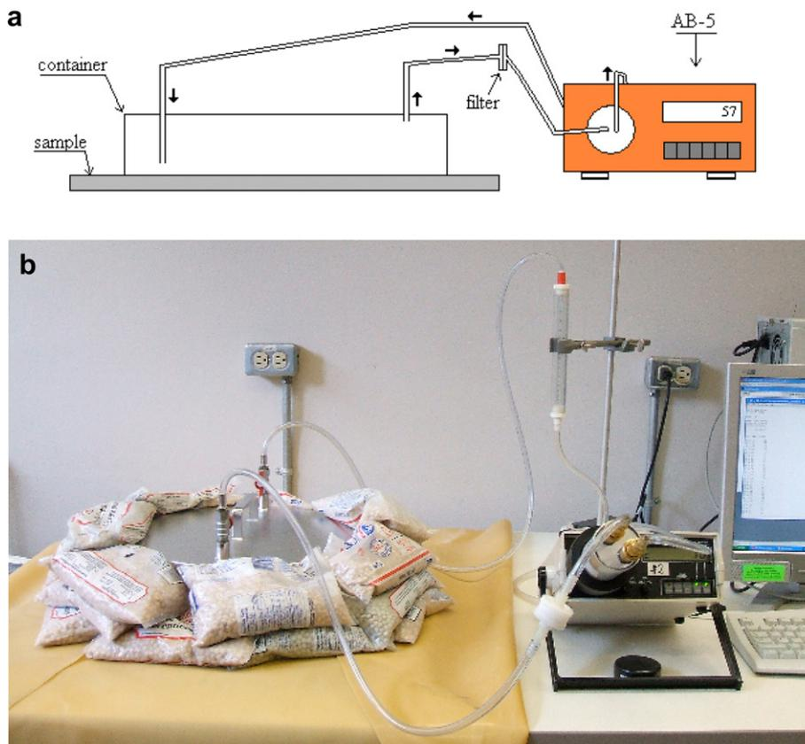
Fig. 1. Experiment set-up for surface radon exhalation measurement, a sketch (a) and a photograph (b).
