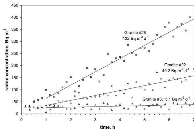
**Fig. 3.** Examples of radon growth curves and the derived radon exhalation rates for Granite #3 ( $5.1 \text{ Bq m}^{-2} \text{d}^{-1}$ ), #22 ( $49.2 \text{ Bq m}^{-2} \text{d}^{-1}$ ), and #28 ( $132 \text{ Bq m}^{-2} \text{d}^{-1}$ ).
